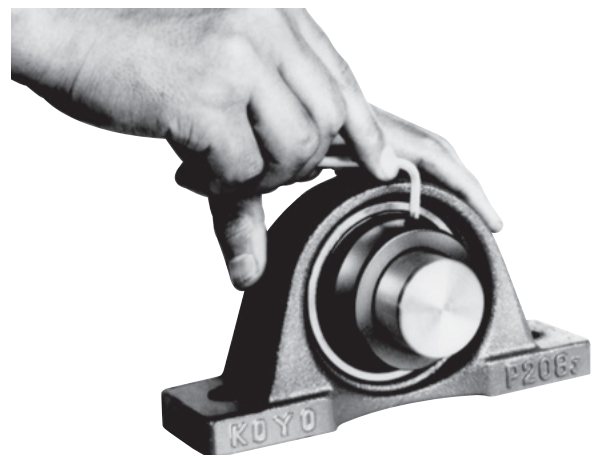
Fig. 14.10 Installing eccentric locking collar
