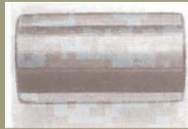
Cylindrical roller with polished surface, due to the scarcity of lubricant.
