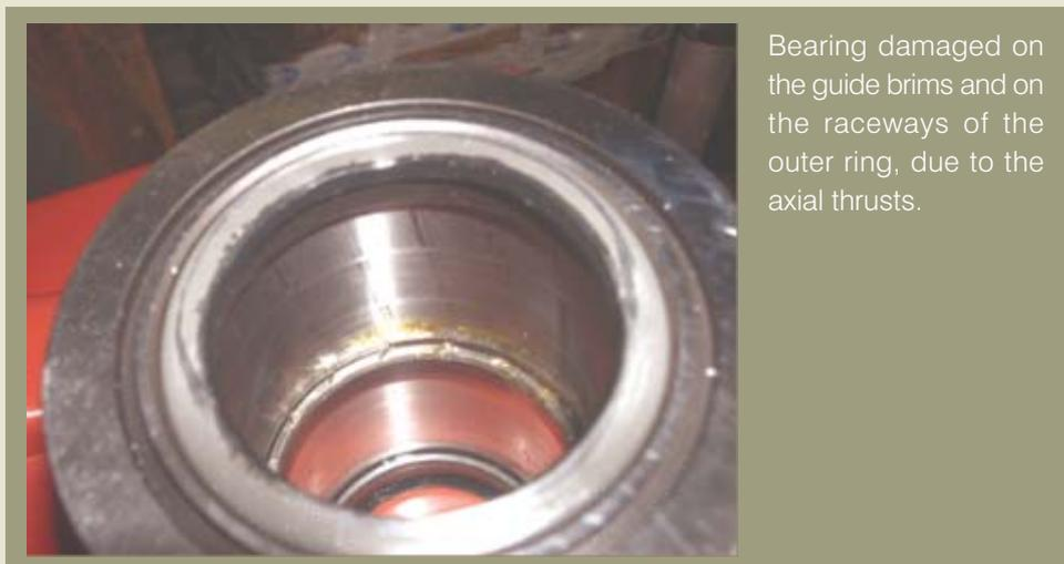
Bearing damaged on the guide brims and on the raceways of the outer ring, due to the axial thrusts.
