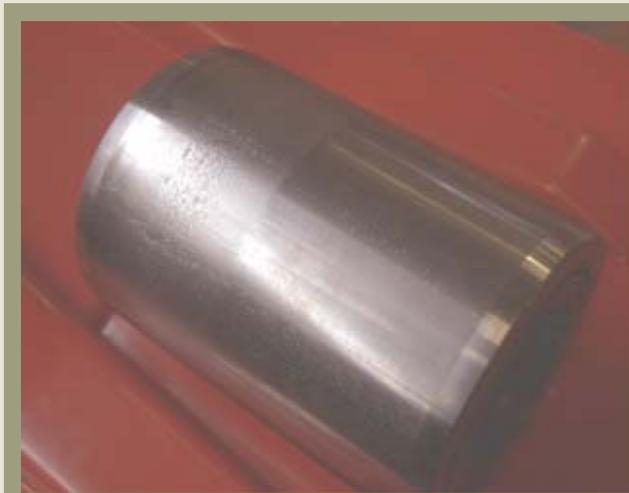
Outer ring with evident marks of wrong functioning, due to a non correct alignment; the part of the outer ring which is not damaged is still polished.
