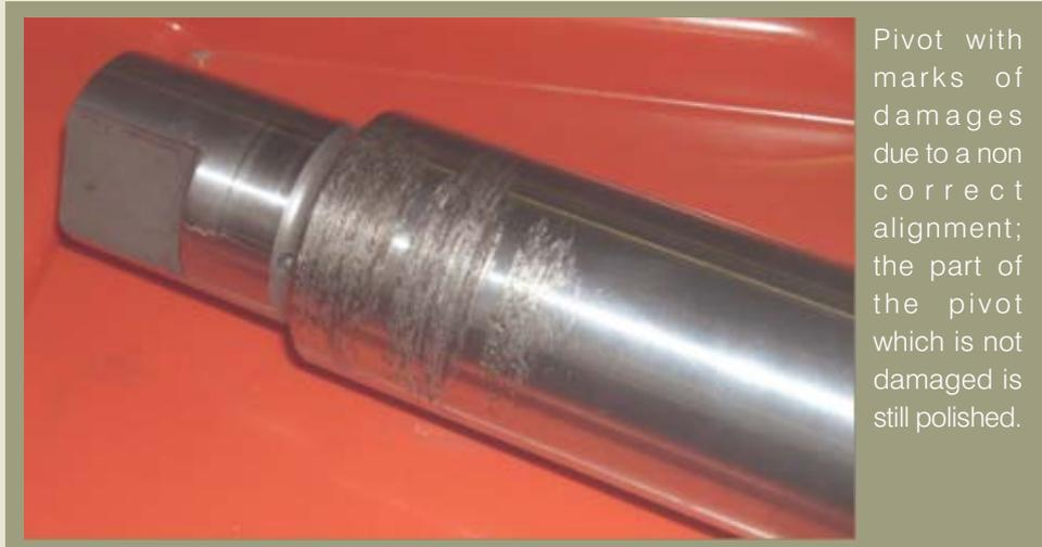
Pivot with marks of damages due to a non correct alignment; the part of the pivot which is not damaged is still polished.
